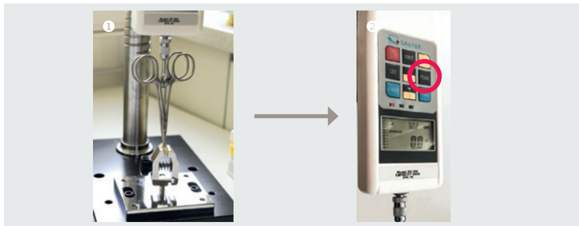
Figure 5. Evaluation of separation force of explants. (1) explants are fixed to a force transducer, (2) maximal force is recorded, which is needed to separate explants.
